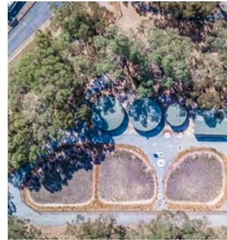
The Waterproofing Eastern Adelaide Project involved the design and construction of a stormwater harvesting scheme to capture, treat, store through an Aquifer Storage and Recovery (ASR) Scheme and then distribute recycled stormwater for irrigation purposes across the
