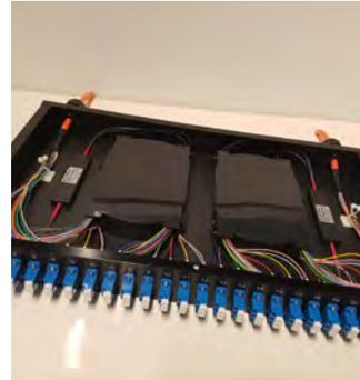
Modular Photonics, a spin out from Macquarie University, manufactures glass-microchip devices that increase data transmission rates and reach in legacy public and enterprise optical fibre networks, and next generation intercontinental and inter-city fibre links. The
