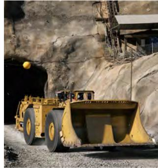
This project was to design, develop, test, validate and bring to market the next generation R1700 Load Haul Dump (LHD) for Underground Hard Rock Mining. This machine will be the engineering and product architecture foundation of a series of new product releases for Caterpillar's Hard Rock
